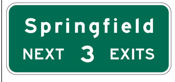
Figure 2E-33. NEXT EXITS Sign
